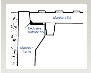
Stop inflow around the manhole lid with our low maintenance lid gasket option for sealing existing manhole lids.
