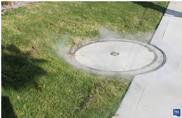
Figure 11 Smoke from under the surround of a MH – I/I source
