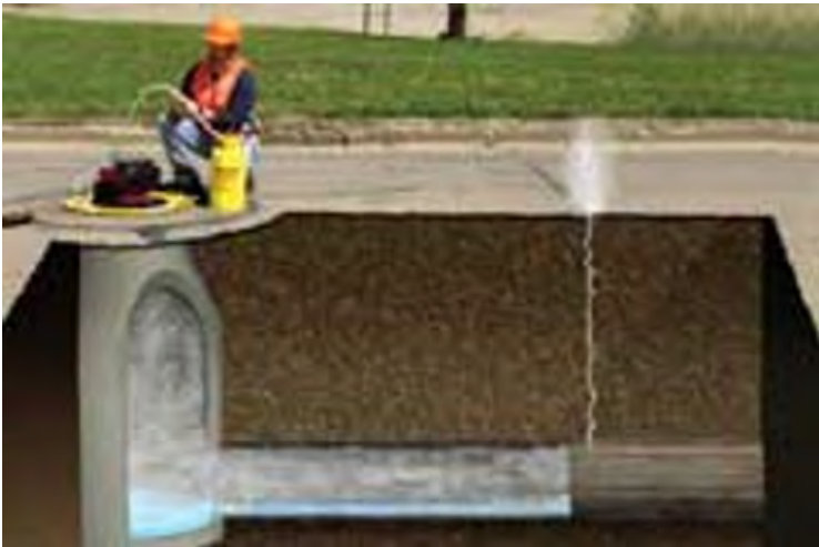
Figure 8 Schematic showing how smoke is introduced at a manhole and shows leaks from a cracked pipe
