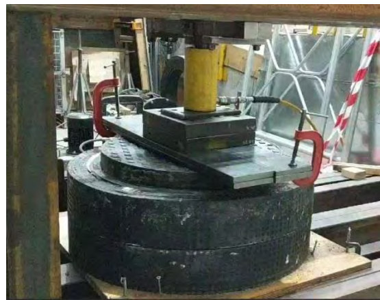
Figure: 7 Subject: Fatigue rig assembly (after lid cracked)
