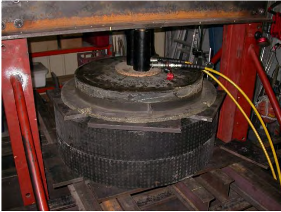
Figure: 4 Subject: Ring assembly load test
