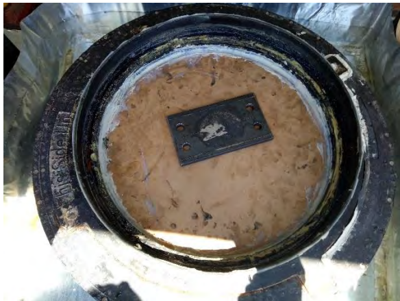
Figure: 6 Subject: Gas tightness test rig with water external (air filled into chamber under wooden seal insert)
