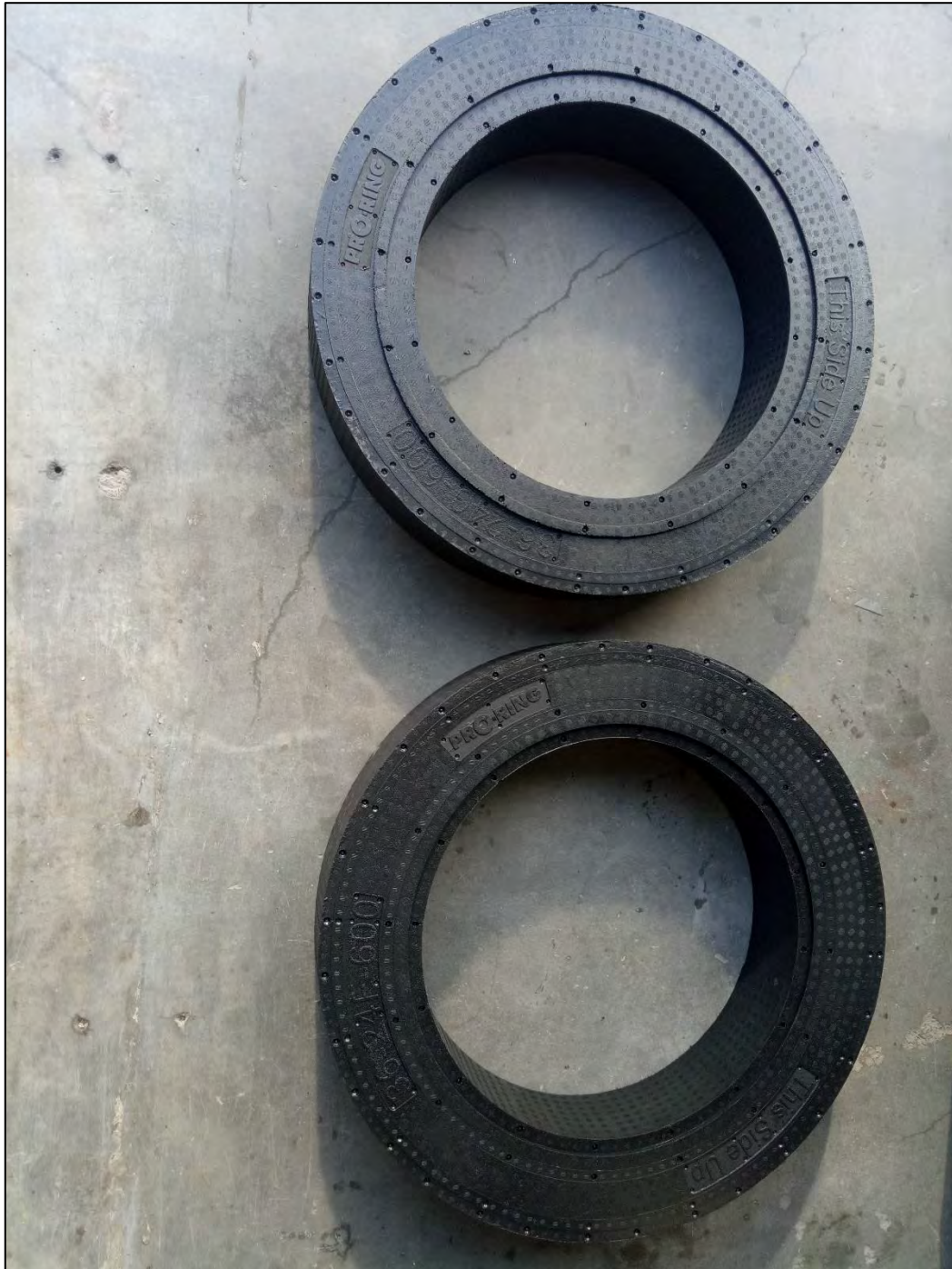
Figure: 1 Subject: Cretex Pro-Ring™ make-up rings submitted for testing
